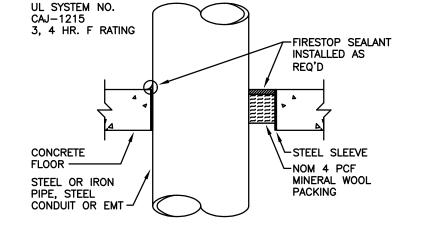
CONCRETE FLOOR OR WALL PENETRATION FIRE-STOP ASSEMBLY DETAILS FOR PIPING & DUCTWORK
