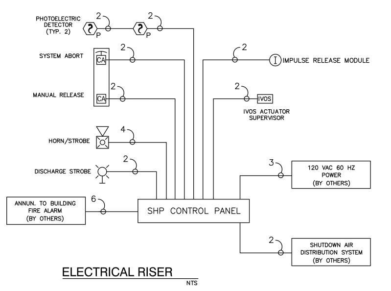
NOTE: ALL WIRING SHALL BE THHN #14 AWG STRANDED UNLESS OTHERWISE NOTED. SEE ELECTRICAL NOTES ON SHEET 2 FOR POWER INPUT WIRING.
