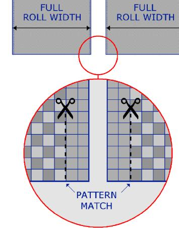
NOTE: THE TRIMMED SELVEDGE OR FACTORY EDGE OF EACH ROLL IS TO BE SEALED WITH THE APPROPRIATE SEAM SEALER PRIOR TO INSTALLATION.
