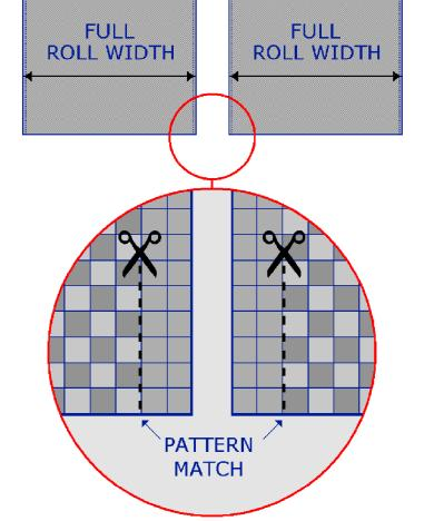
NOTE: THE TRIMMED SELVEDGE OR FACTORY EDGE OF EACH ROLL IS TO BE SEALED WITH THE APPROPRIATE SEAM SEALER PRIOR TO INSTALLATION.
