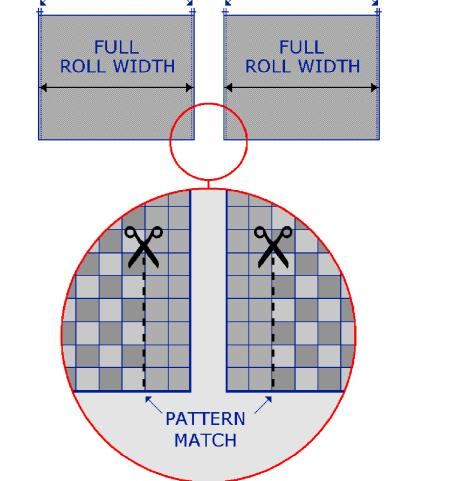
NOTE: THE TRIMMED SELVEDGE OR FACTORY EDGE OF EACH ROLL IS TO BE SEALED WITH THE APPROPRIATE SEAM SEALER PRIOR TO INSTALLATION.
