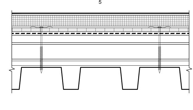
ROOF TYPE A BARREL R-20 (MINIMUM R-VALUE 20)
