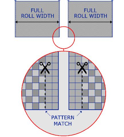
NOTE: THE TRIMMED SELVEDGE OR FACTORY EDGE OF EACH ROLL IS TO BE SEALED WITH THE APPROPRIATE SEAM SEALER PRIOR TO INSTALLATION.
